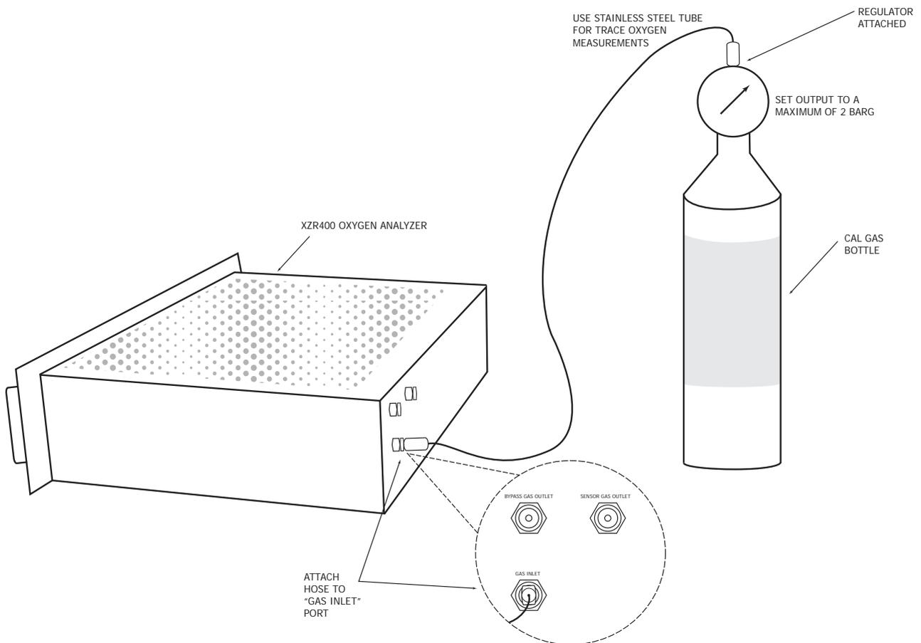
Figure 44 Calibration Procedure with XZR400A1
