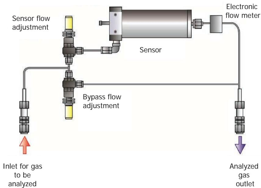
Figure 19 Gas Circuit Diagram for XZR400A2, A3 & A4 models
