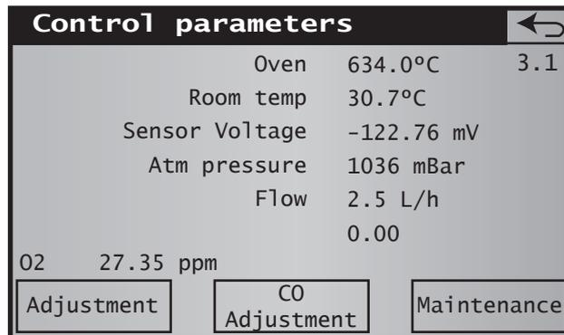
Figure 33 Control Parameters Screen
