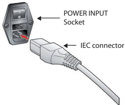
Figure 28 *Power Input Socket*
