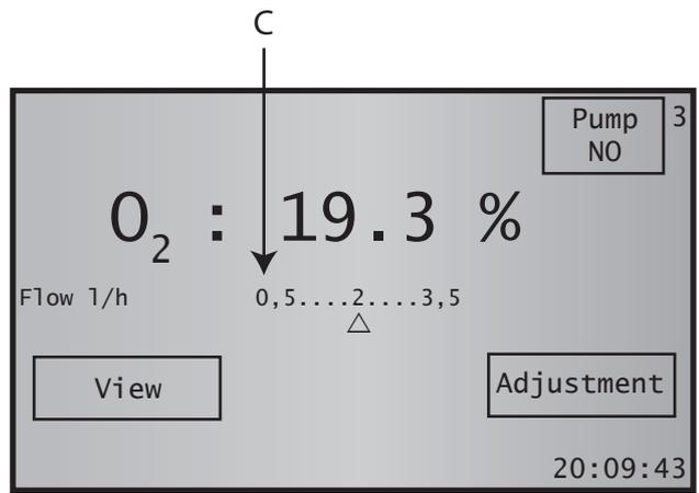
Figure 31 Sample Flow Adjustment
