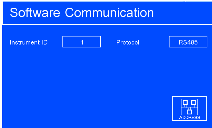
Figure 37 Software Communications Screen
